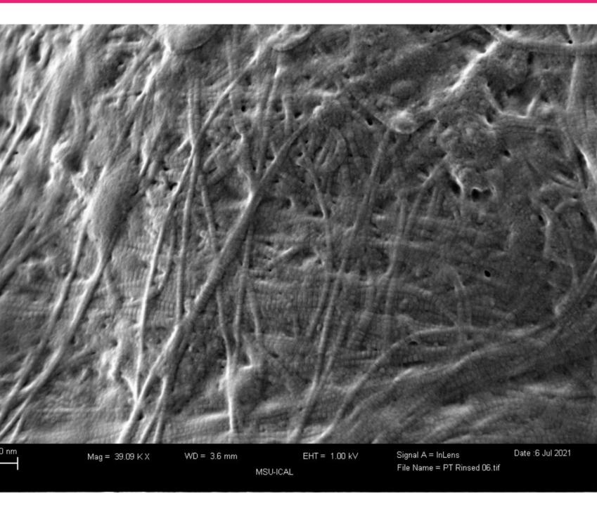
**Figure 5.** SEM micrographs of post-processed umbilical cord tissue samples. SEM image of preserved cross-linked collagen structures. (Scale bar: 300nm). Average iber diameter, 65.4 nm.
