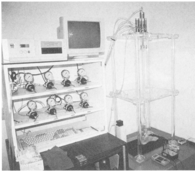
FIGURE 3 Testing apparatus consisting of custom load frame and actuator controls with specimen in place.
